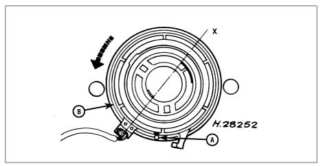
31.5 Centring the air bag clock spring. Depress locking pin (A) and rotate outer rotor (B) anti-clockwise ("X" indicates relative position of the direction indicator cancelling cam to the cable connector - see text)
